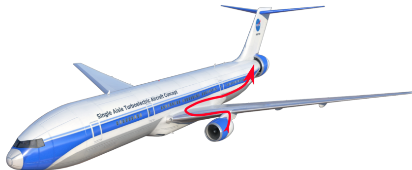
Figure 1.8: The STARC-ABL configuration, with the turboelectric power flow highlighted by the red arrow. Electric power is generated by generators on the underwing nacelles and send to the aft fuselage to power an electric BLI propulsor.
