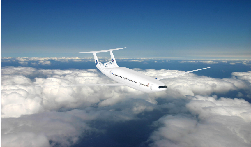
Figure 1.2: Artist conception of a notional D8 aircraft concept with top, aft mounted BLI propulsion system.
