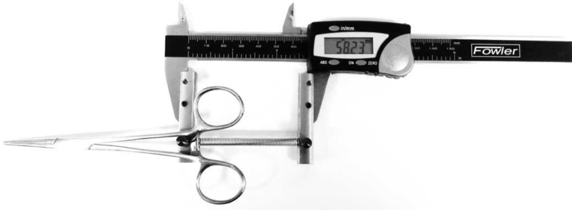
Figure 2.3: A calibrated spring stretched across the jaws of a digital readout calipers enables the determination of tension applied to produce a specified displacement of the incision edge. Force is applied to the proximal caliper jaw by hand and to the distal jaw by the locking needle driver secured to the abdominal fascia.
