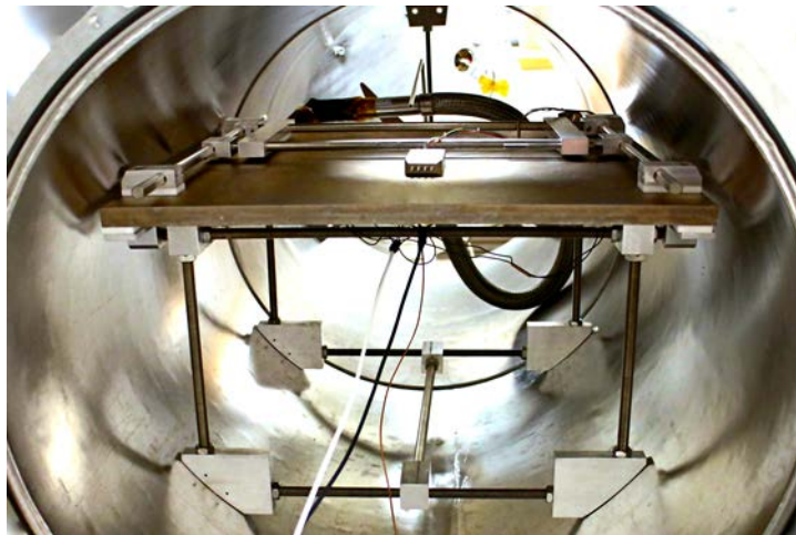
Figure 6.2: The Michigan Mars Environmental Chamber is capable of simulating Martian polar conditions, covering the environmental conditions found at the Phoenix landing site that were not tested during preflight tests. The TECP Engineering Model is sitting on top of thermal plate to allow thermal contact.
