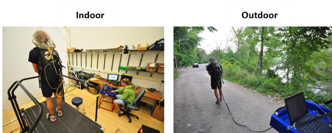
Figure 3-2. Indoor and outdoor environments. Left panel shows an example subject standing on the instrumented, split-belt treadmill in front of the projector screen displaying the indoor, virtual environment. Right panel shows an example subject walking along the outdoor path tethered to an experimenter by cables from measurements devices connected to a laptop on a tray.
