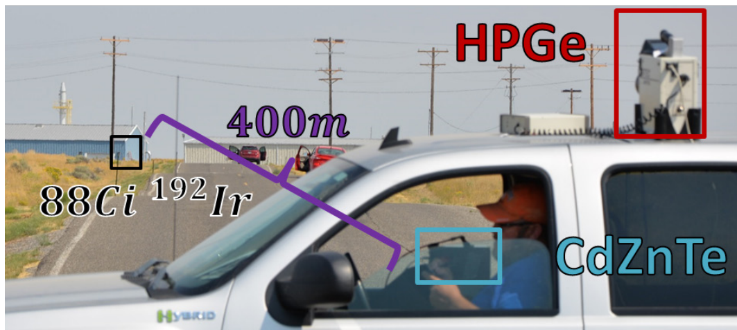
Figure 4.2: (Top) Measurements were conducted at Idaho National Laboratory with a pickup. The CdZnTe system was placed inside the truck cab. Sources were on top of a 3.5 m ladder well away from buildings to mitigate scatter. The truck cab window facing the source was opened giving the CdZnTe system an unimpeded view of the source. Source location is highlighted with a black box with the inset figure showing additional detail. (Bottom) Far-field measurement at 400 m showing relative HPGe placement on the truck roof.
