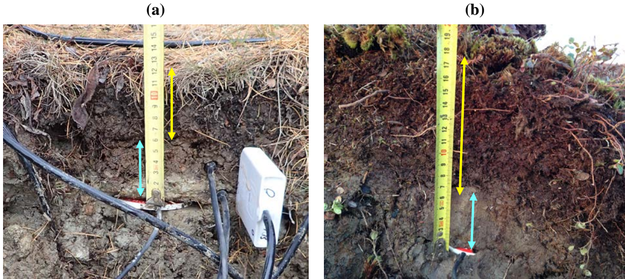
Figure E1: An example of installation of heat flux plate at the depth of 6 cm (cyan arrow) below the top of mineral soil in the Polar Urals, Russia. (a) The thickness of the ‘O’ horizon and peat layer (yellow arrow) containing undecomposed and partially decomposed organics is ~6 cm. (b) For a different site with the same instrumentation setup, the peat thickness is ~12 cm, also containing a surface moss layer. Soil temperature sensors at the depths of 2 cm and 4 cm (black cables) as well as averaging soil moisture and temperature sensor at the same depth range (white plastic head) can be seen to the right of the heat flux plate in (a).
