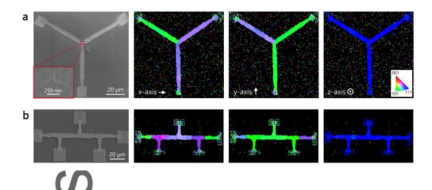
**Figure 4.** Preparation of tricrystals and bamboo-like morphologies that extend the growth platform beyond bicrystals. a) SEM image and EBSD maps in the z-, y-, and x-sample-axes for tricrystals, which are specified by Y-shaped microstructures; the platinum-mediated crystal growth process drives the formation of a triple junction (inset). b) SEM image and EBSD maps in the z-, y-, and x-sample-axes for bamboo-like gold interconnects prepared by defining branches with multiple seeds.
