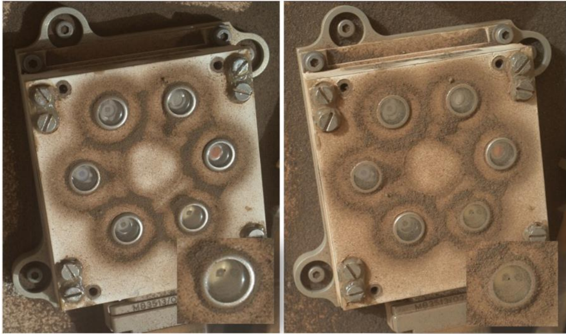
Figure 1: Dust deposition on the UV sensor: comparison between MSL sols 2036 (pre-storm) and 2216 (after the storm), taken by MAHLI. The images were taken at different times of sol, hence with different sun position, as evidenced by the different sun glint locations at the edges of the photodiodes. It can be seen in the zooms for both images of the same photodiode that the sensor is almost blocked by the dust, which highlights the deposition of dust over the rover due to the dust storm.
