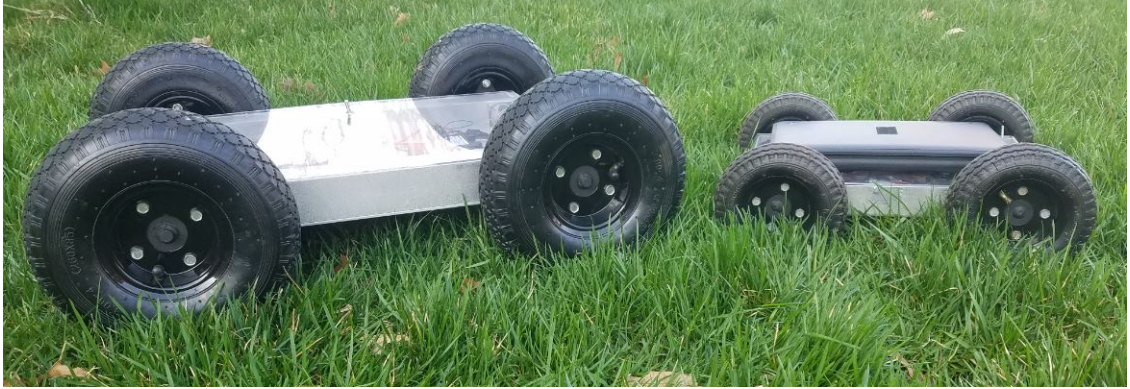
Figure 3.2: Large (10 inch wheels and 15.15kg mass) and small robots (6 inch wheels and 7.25kg mass) used for experiments.
