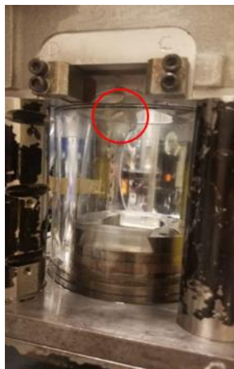
Figure 3. 4 Combustion chamber of the optical engine. Optical collector was directed towards the area marked with the red circle.
