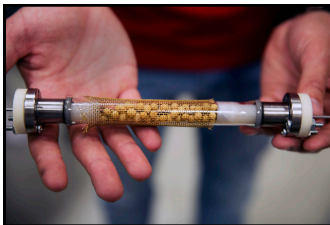
Figure 1-2: An image capturing the 3-dimensional packed bed reactor filled with soybean aggregate.
