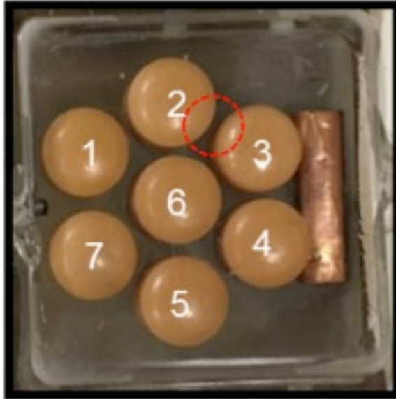
Figure 4-9: Image representing the second location of investigation between dielectric aggregate labeled 2 and 3.
