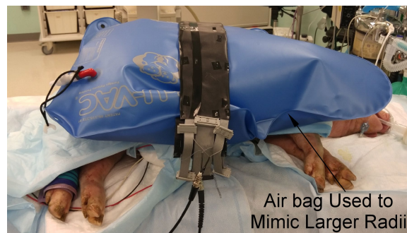
Fig. 5.43: Inflated airbag is inserted between the subject and the coils for mimicking larger waist patients.
