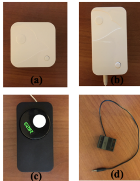
Figure 2-3 Sensors and Probes for Indoor Environment Data Collection (a) Gateway; (b) Temperature and humidity sensor; (c) CO 2 probe; (d) Window contact probe
