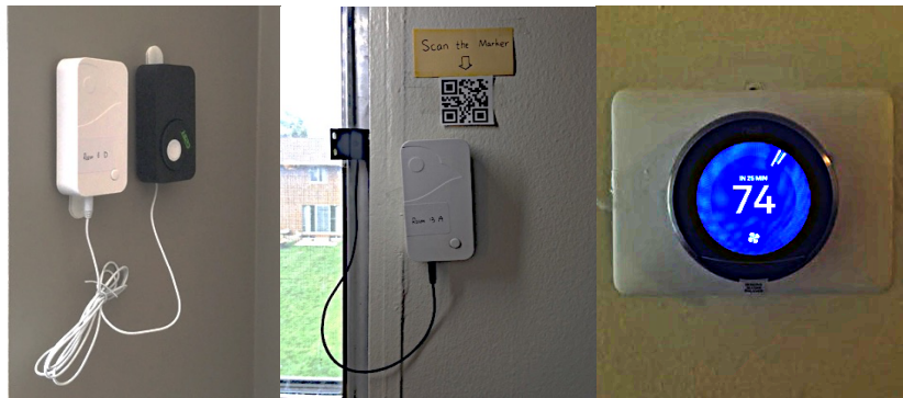
Figure 2-9 Temperature and CO 2 Sensors (left); Location Marker and Window Sensor (middle); Nest Thermostat (right)
