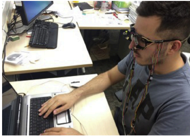
Figure 3-3 Eyeglass Frame with Infrared Thermometers (adapted from Ghahramani et al. 2016)
