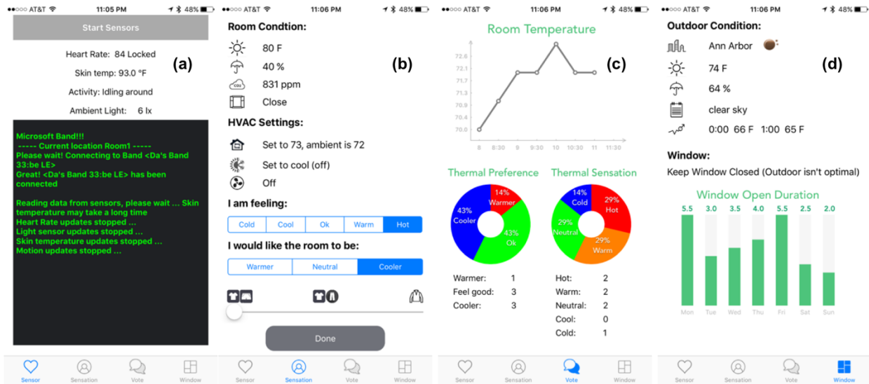
Figure 2-6 Application Interfaces for (a) Human physiological data; (b) Thermal sensation and preference; (c) Collective opinion; (d) Conditioning mode
