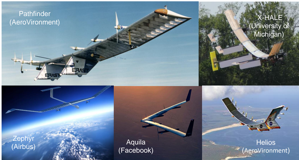
Figure 1.1: Examples of HALE aircraft: Pathfinder (AeroVironment), Zephyr (Airbus), Aquila (Facebook), Helios (AeroVironment) and X-HALE (University of Michigan). Propellers are usually a propulsion choice for such light and low speed configurations
