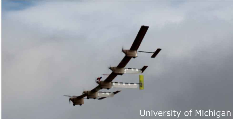
Figure 5.3: 6-m span X-HALE vehicle in flight
