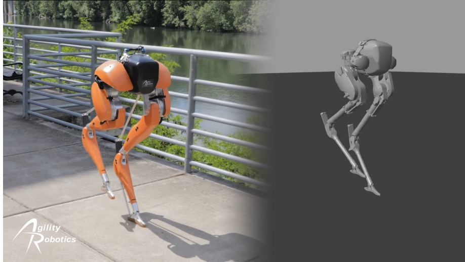
Figure 7.1: The bipedal robot Cassie (left) and a realistic model (right). Image taken from the video Cassie Sim Comparison released by Agility Robotics [80].
