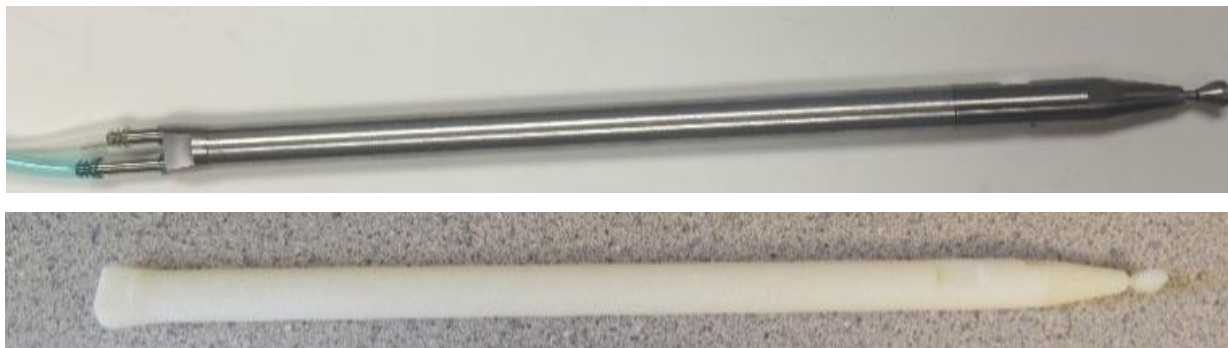
FIGURE 23: Insertion wand and model (top) Actual insertion wand, with pneumatic hoses on the left and actuating head on the right. (bottom) 3D printed model. Model length is 17.1 cm.
