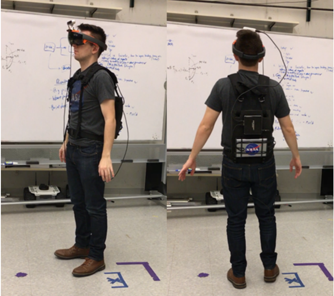
Figure 3.5: Subjects wear a harness with an Intel NUC and power bank attached to their backs. The NUC processes data from the Intel RealSense depth camera as well as the Pupil Labs eye trackers. Both sensors are fastened to a Microsoft HoloLens worn on the users head.
