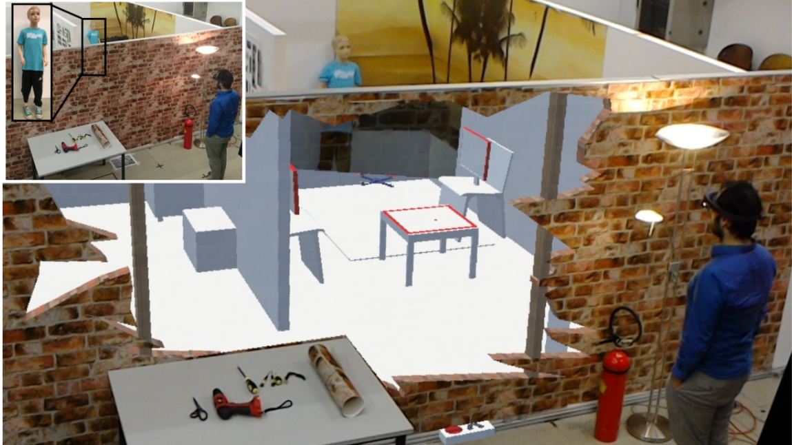
Figure 1.14: In [14], a human was tasked with piloting a UAV, via gaze inputs, through an occluded environment. This was done by projecting exocentric views of the environment onto the obstructing wall with AR. Thus, the human was given virtual x-ray vision.
