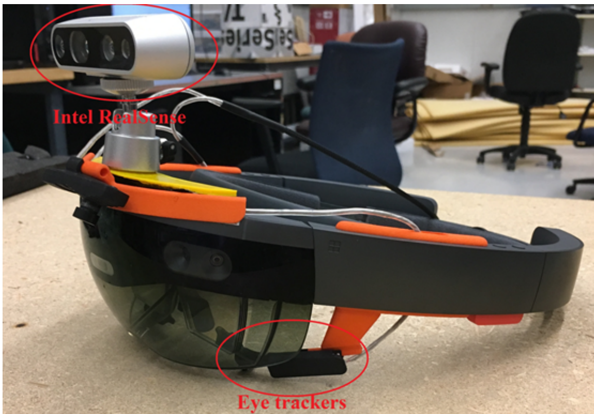
Figure 3.4: Subjects wear a Microsoft HoloLens over their eyes to view the UAV's camera feed. Their gaze is tracked via Pupil Labs eye trackers and the point cloud \mathcal{P} is gathered via an Intel RealSense depth camera.
