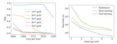
(a) True positive rate. The density varies from 1000– 2000 cars per hour and the discrete grid size changes from  $1m^2-5m^2$ . (b) Runtime of Ubi. We measured the run time for different resolutions  $1m^2-5m^2$ .
