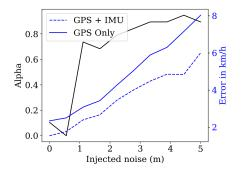
Figure 3.5: Vehicle speed estimation error for increasing high-frequency GPS noise. For higher GPS noise, **CarSec** relies more and more on the accelerometer component of the complementary filter.
