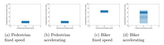
Figure 4.8: Mobility models for 4 different hazard types. Each scatter plot represents the full range of possible movement in one time step with the hazard starting at (0,0). We also compared these with a stationary obstacle that isn't shown here.
