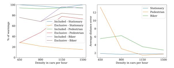
Figure 4.11: Accuracy and distance errors for varying density of cars. "Included" results show the responses which included multiple hazards, including the correct hazard. "Exclusive" results show the responses which only warn the driver about the correct hazard.
