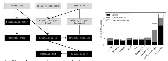
(a) The architecture of our **CarSec** implementation. The gray modules contribute to the estimated outputs. The black modules are the six estimators.
