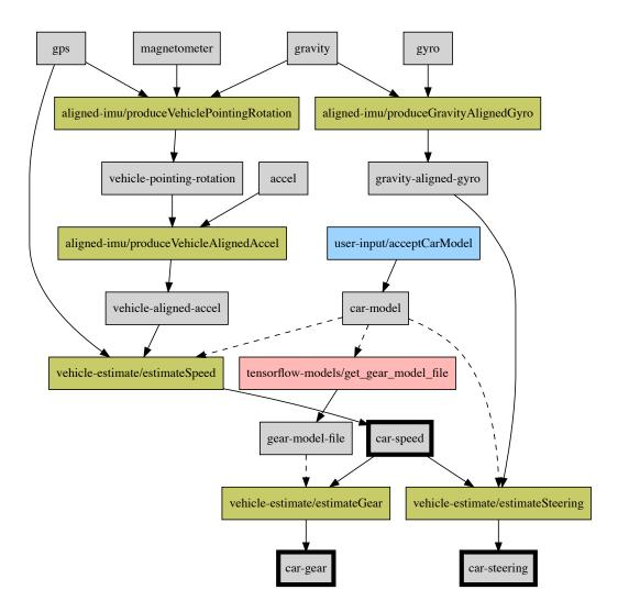
Figure 5.7: All information and algorithms compiled together for a vehicle sensor estimation case study. All information blocks are in gray. The input required information are the three gray blocks with a thick border. The remaining dependencies and all algorithms were determined by CAB's graph search.
