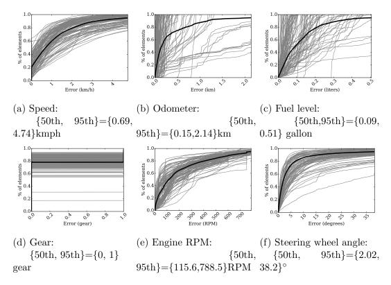
Figure 3.3: Estimation error of vehicular sensors using CarSec. Each CDF shows the estimation error of each trip along with the average error in a thick black line.
