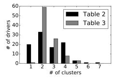
Figure 2.10: Histogram of how many clusters we found for each of the contexts specified in Table 2.4. For each driver, we collected all 10 second time windows for their trips and ran DBSCAN on the final aggregate plot. We used epsilon between clusters = 0.3 and minimum samples within each cluster = 50
