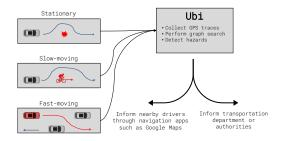
Figure 4.1: Ubi detects different driving hazards (shown in red) by collecting GPS trajectories of vehicles around the hazard (shown in blue). This operation is done in a cloud service and broadcast back to the drivers, or to the proper authorities
