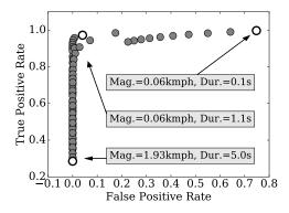
Figure 3.10: ROC curve of 100 different combinations of the two parameters — attack magnitude and duration. For each combination, we calculate the FPR and TPR. A similar ROC curve was computed for each of the 6 sensor estimations.
