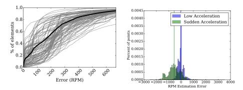
(a) Engine RPM estimation error using the ground truth vehicle speed and gear position.(b) Distribution of RPM errors. Figure best seen in color.
