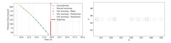
Figure 4.9: The left figure shows the distance from the hazard. Vertical lines show the time of the sightings of the hazard by all cars in the simulation, which is also reflected in the right figure to show the *location* where the sighting took place. The colored scatter points on the left figure represent Ubi's response to the driver, showing both the classification and the distance to the hazard.
