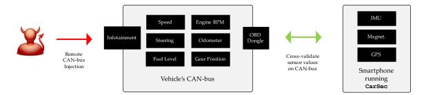
Figure 3.1: Three smartphone sensors are used to infer six different vehicular properties. CarSec compares these inferred values with those reported by the vehicle to detect *sensor-falsification attacks*.
