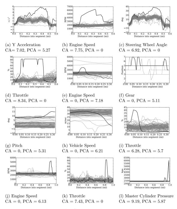
Figure 2.16: Example anomalies for each road segment and each technique. The anomalous trip is highlighted in bold. The sensor and the anomaly scores are listed under each sub-figure.
