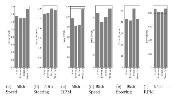
Figure 3.4: Estimation error using the passenger's phone. The black horizontal line shows the 50th and 95th percentile errors for each of these sensors when the phone is more carefully mounted, as done in our previous experiments.
