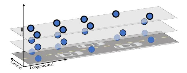
Figure 4.5: The open space around the GPS trajectories are represented using a network. Each node represents a potential location for the hazard.
