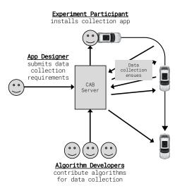
Figure 5.1: Three parties involved in CAB. Algorithm developers contribute code to the CAB repository. App designers, which could be researchers or app developers, submit high-level requirements. The CAB server takes the available algorithms and automatically compiles a data-collection app. The *Experiment participant* joins the data collection and installs the data-collection app
