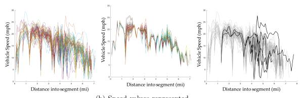
(a) Aggregated speed values over the same road segment. (b) Speed values represented using the top principal component. (c) Anomalous speed values highlighted in black.
