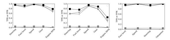
(a) Sudden attack where the (b) Gradual attack where (c) Delta attack where the atattacker immediately sets the the sensor value gradually tacker sets the injected value sensor value to the target changes to the target over a to a offset of the value. span of 10 seconds. actual value.
