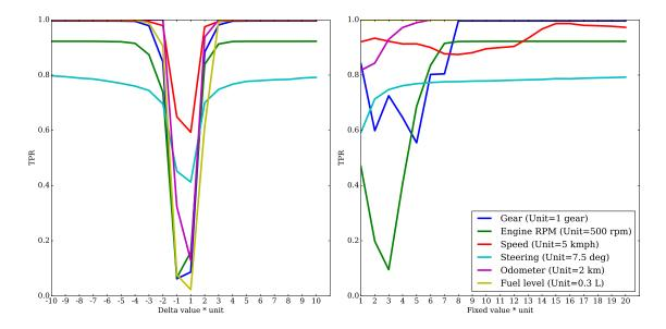
Figure 3.11: The left figure shows TPR for varying amounts of injection magnitude. The right figure shows varying *fixed* values of injection. At the moment of the injection the vehicle sensor varies depending on the scenario. For instance, in some cases the car was traveling at 10 kmph when there was a 4kmph injection. For all cases, FPR was less than 5% and therefore omitted. Figure best seen in color.
