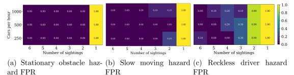
Figure 4.13: Heatmap of false positive rate for each hazard type. The number of sightings varied from 1–6 and the density of cars changes from light (250 cars per hour), medium (500 cars per hour) and dense (1000 cars per hour).
