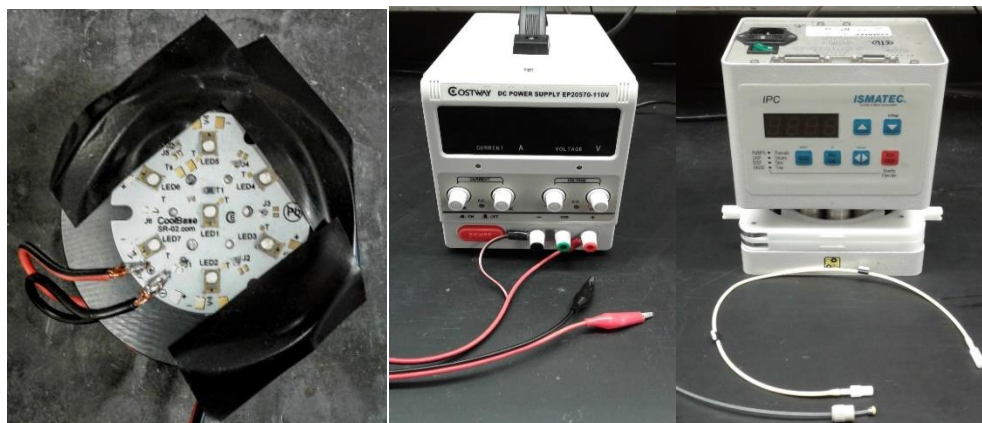
Figure 2.13. Continuous flow processing equipment (Left: Luxeon SP-02-V4 Royal Blue LED mounted to heat sink; Middle: Ismatec peristaltic pump; Right: Costway DC controller)
