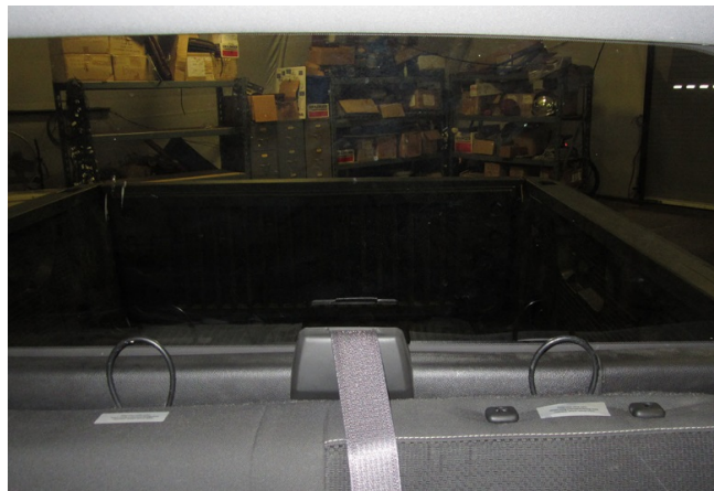
Figure 1. Chevy Silverado (vehicle 1) uses plastic-coated wire tether routers/loops.
