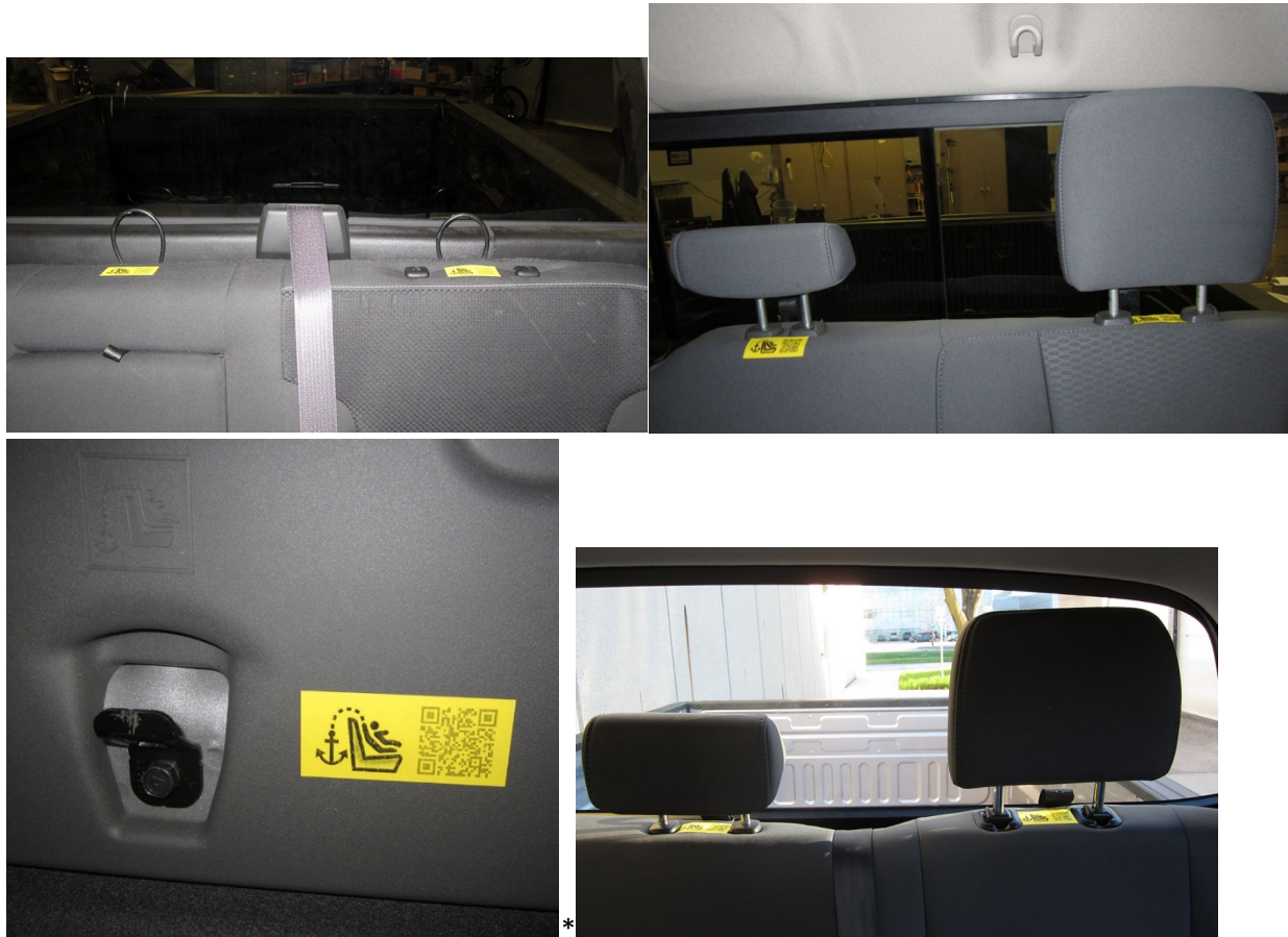
Figure 13. Information on QR code label and labels installed in vehicles (Silverado top left, Ram top right, Frontier bottom left, Tundra bottom right.)
