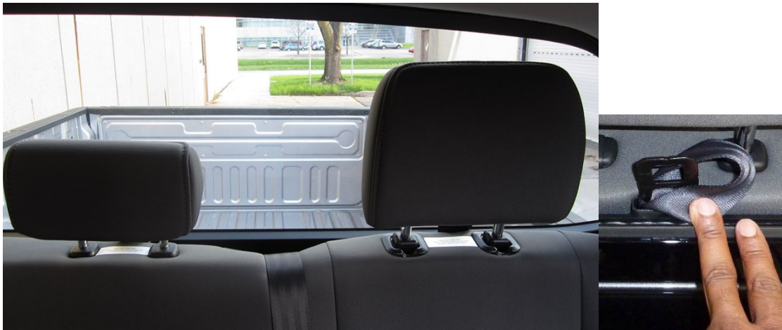
Figure 4. Toyota Tundra (vehicle 4) uses webbing routers and metal anchors.
