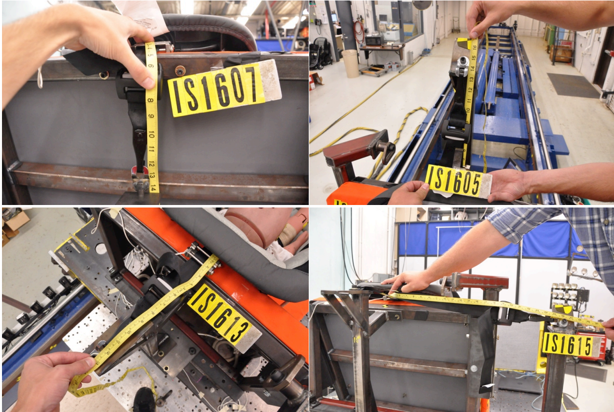
Figure 19. Tether anchor conditions, clockwise from upper left: down, up, back and adjacent.
