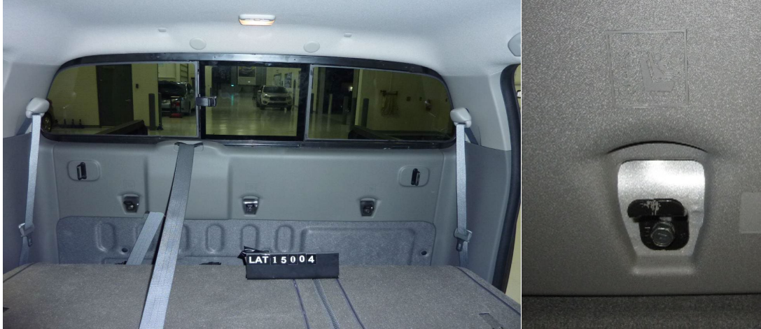
Figure 3. Nissan Frontier (vehicle 3) uses metal tether anchors attached to back wall of cab behind vehicle seat.
