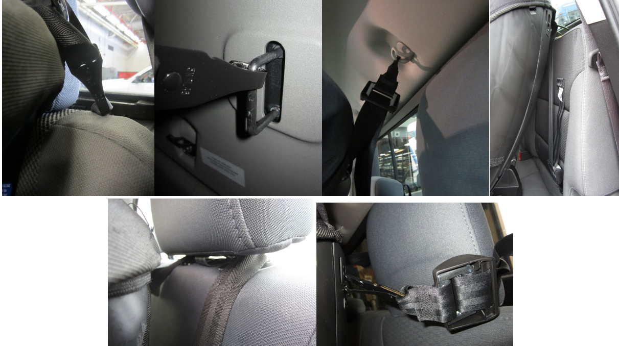
Figure 15. Examples of incorrect attaching to non-tethers: seat adjuster, cargo hook, storage hook, lower anchor, around head restraint, child restraint storage hook.
