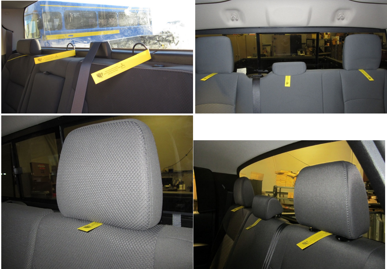
Figure 7. Tether tags in each vehicle (Silverado top left, Ram top right, Frontier bottom left, Tundra bottom right.)
