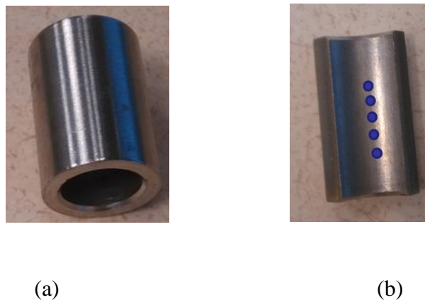
Figure 2.8. Tube samples: (a) a one-inch long short section cut from our received Incoloy 800 H/HT tube and (b) cut-open tube piece from (a)
