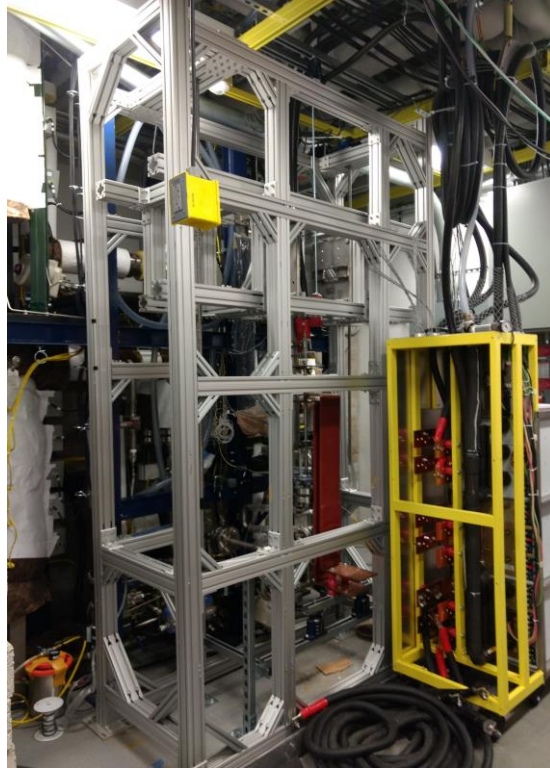
Figure 2.42 Platform to traverse the X-ray radiography system and gamma densitometer
