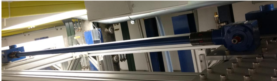
Figure 2.43 Screw jack system on top of the T-slot beam structure
