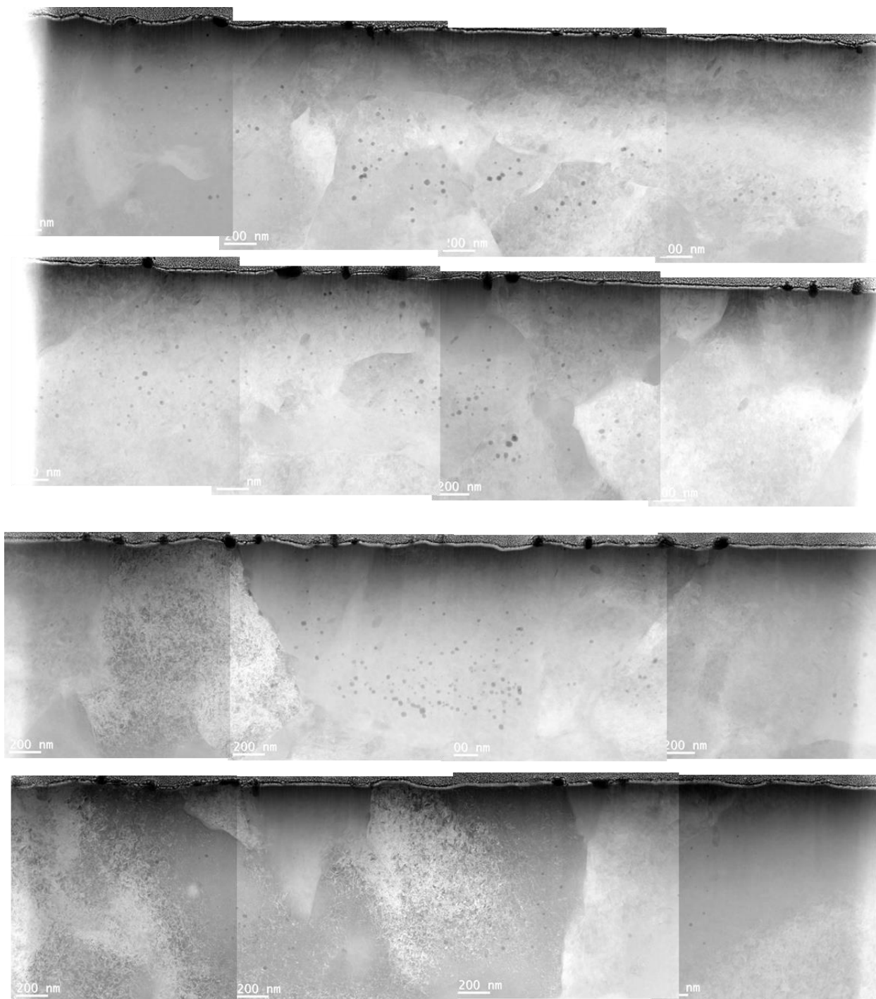
Figure B.13: STEM HAADF Images for liftouts from the irradiation of T91 at 445°C with 0.02 appm He/dpa to 100 dpa.
