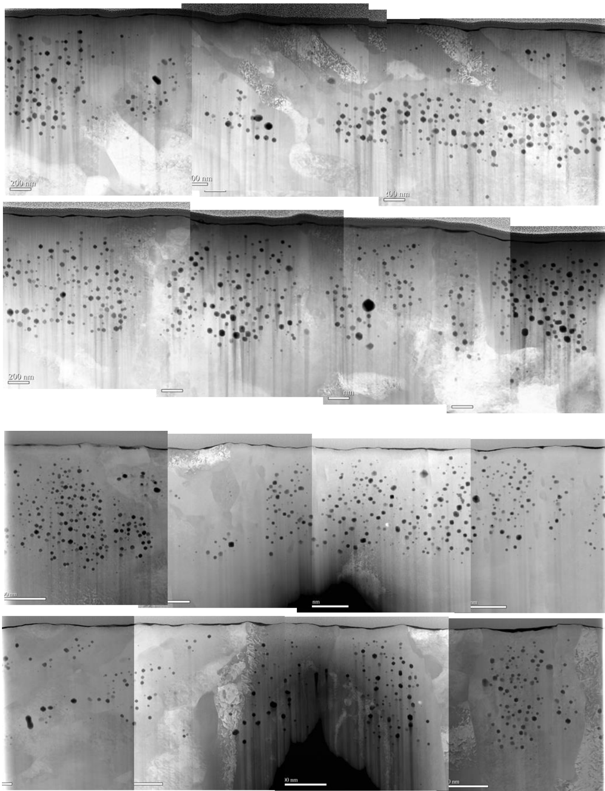
Figure B.5: STEM HAADF Images for liftouts from the irradiation of HT9 at 460°C with 4 appm He/dpa to 350 dpa.
