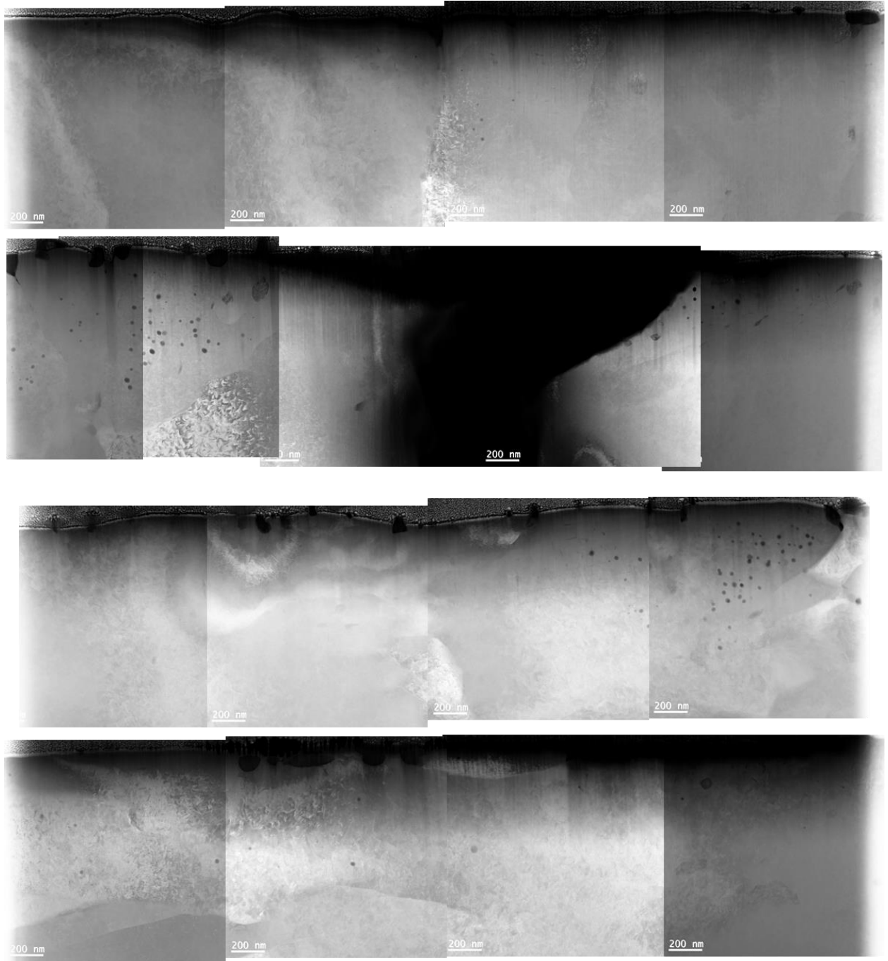
Figure B.20: STEM HAADF Images for liftouts from the irradiation of T91 at 445°C with 4 appm He/dpa to 150 dpa.
