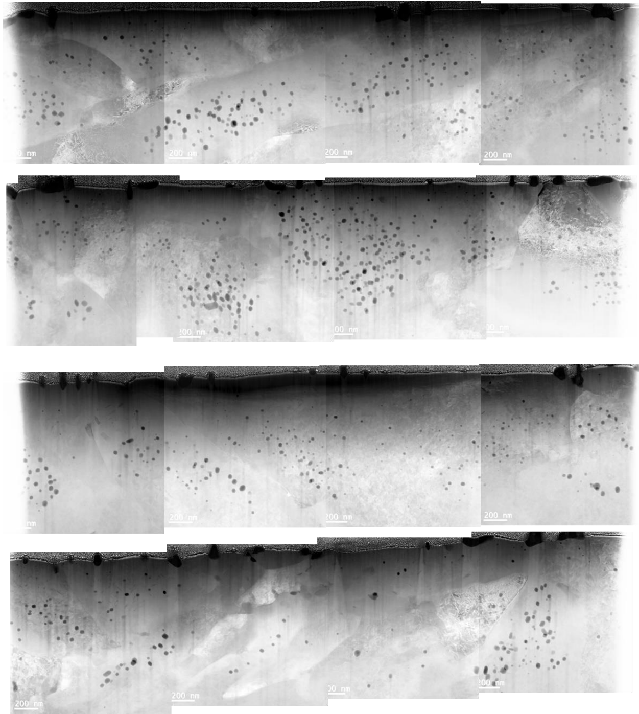
Figure B.16: STEM HAADF Images for liftouts from the irradiation of T91 at 445°C with 0.2 appm He/dpa to 150 dpa.
