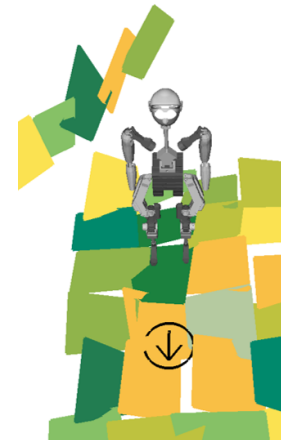
Figure 6.4: Left: All categories of the contact transitions. The inner or outer foot means the foot in the same or opposite side of the palm contact. Each dimension includes all the initial contact poses, the new contact pose (if there is any), and initial CoM position and velocity. Right: An example environment to collect the training data. The tilting angle of each surface, the wall orientation, and wall distance to the robot are randomly sampled.
