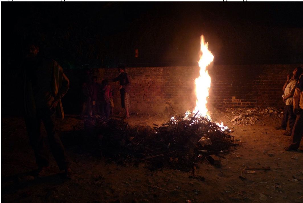
Figure 10 Burning a heap of wires to recover the copper inside
