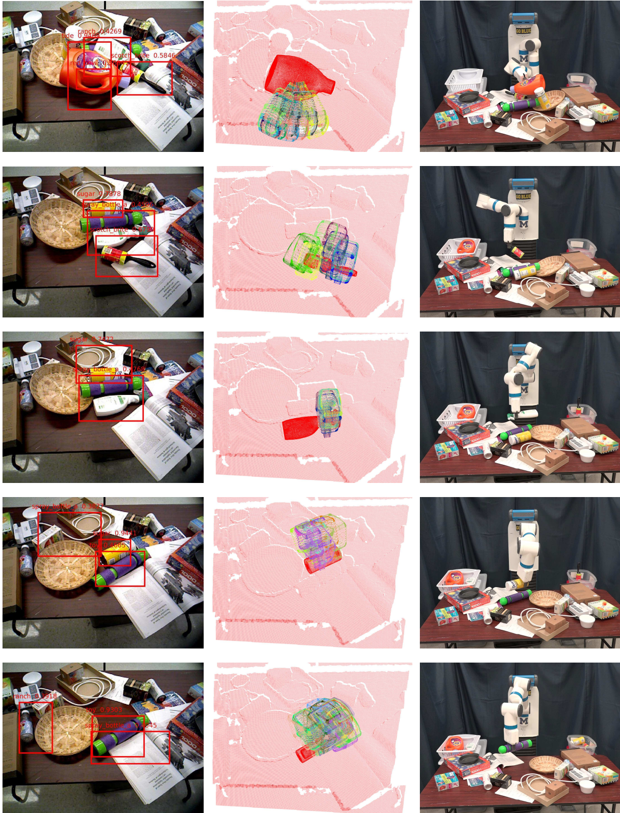
Figure 4.7: Sequential manipulation by a robot to sort 5 objects on a cluttered tabletop into two bins: cleaning (right bin) and non-cleaning (left bin). From the left to right is the detection results from RCNN object detector, most likely object from SUM , computed collision-free grasp poses and robot manipulating the object in action. Our system estimated and manipulated “tide”, “scotch brite”, “sugar”, “toy” and “spray bottle” sequentially.
