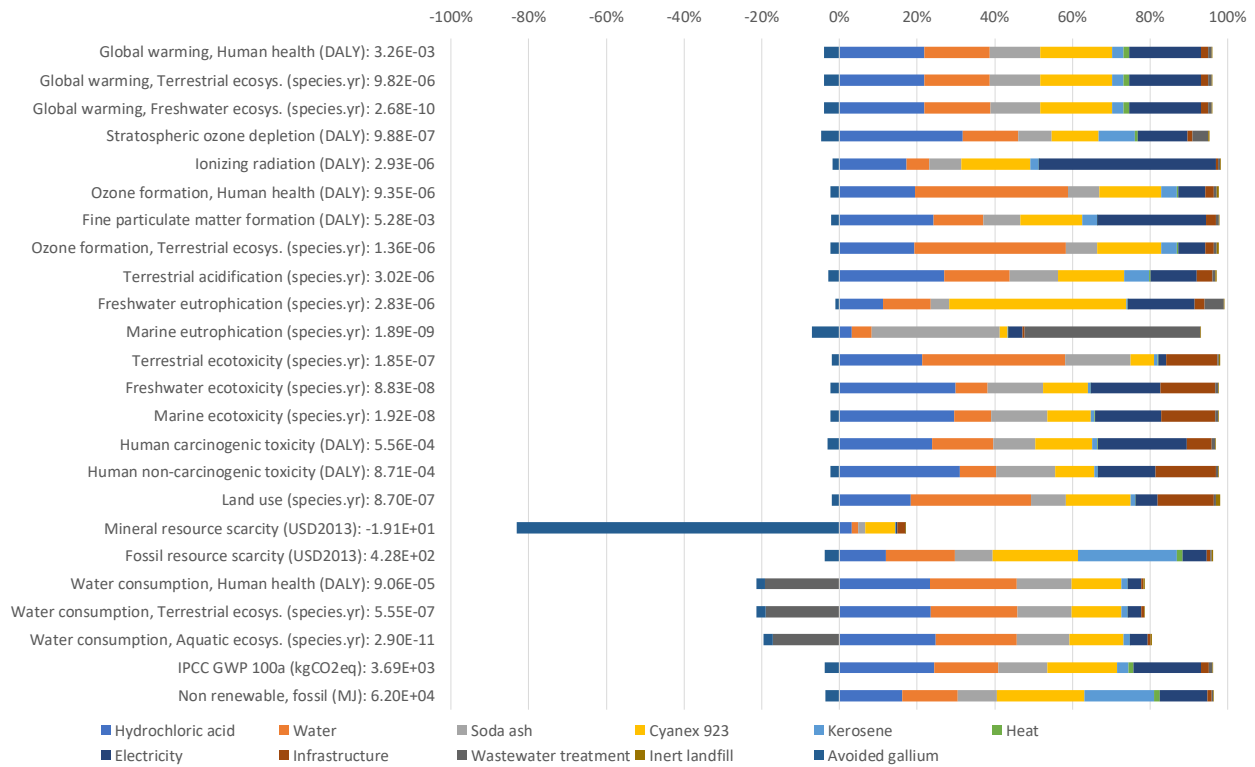
Figure 4.5: Environmental impacts per 1 kg gallium recovered from the LED fraction of linear LED lamp waste via leaching and solvent extraction.
