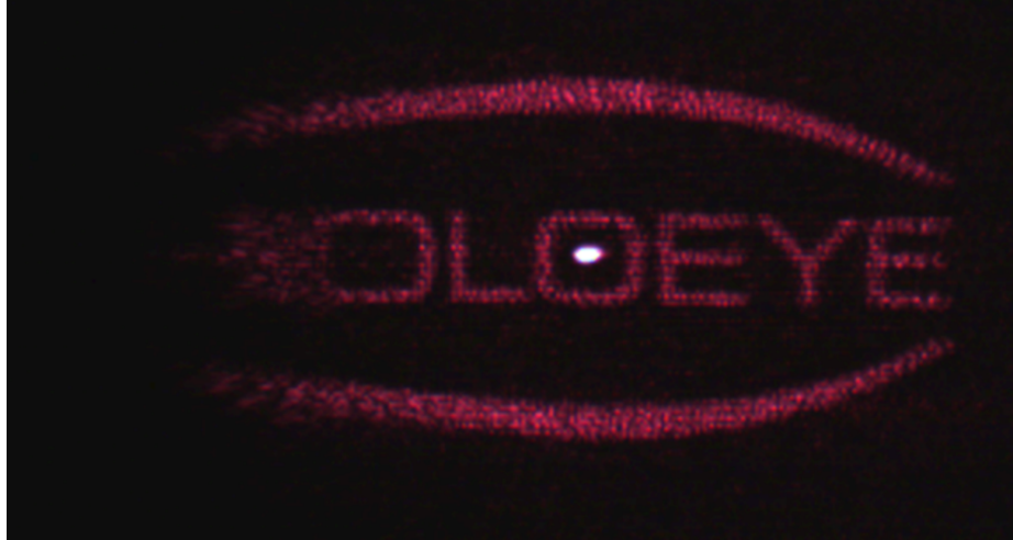
Figure 3.9: The Holoeye logo produced using the zeroth-order reflected beam from a SLM programmed with a CGH coded with the Fourier transform of the image. The bright spot at the center is the unmodulated component of the reflected beam and demonstrates the disadvantages of using the zeroth-order signal.
