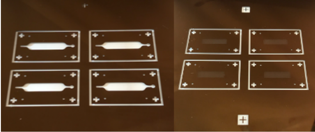
Figure 4.1: Photographs of the microfluidic masks. These masks are used during contact lithography to cure SU-8 in the illuminated pattern. The masks on the left is the first layer, which consists of the canal. The pattern on the right contains the array of triangular microwells that are used to capture the cells.
