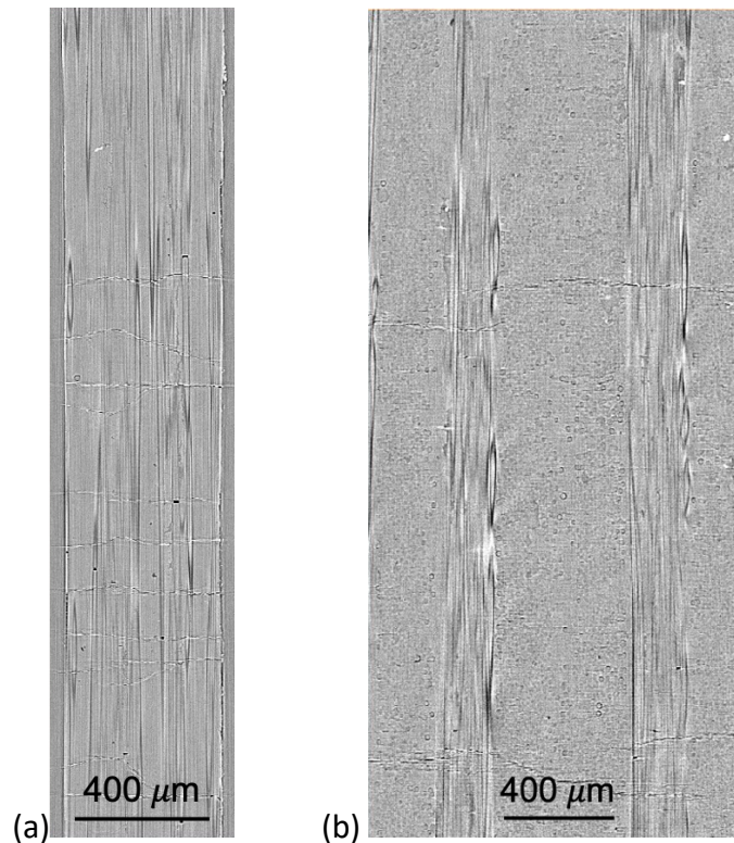
Figure 1.1 2D slices taken within the 3D volume of (a) a unidirectional specimen with fibers running parallel to the loading direction 0^\circ and (b) 2D image of a cross-ply specimen [0^\circ/90^\circ]_s symmetric around a matrix rich region. There are a total of 8 plies with alternation 0^\circ/90^\circ plies with the 0^\circ degree plies parallel to the tensile loading direction and the 90^\circ degree plies perpendicular to the loading direction
