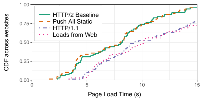
Figure 2.3: Estimation of page load time improvements that would be enabled once HTTP/2 is globally adopted. Given that the adoption of HTTP/2 is still in its nascency today, the fidelity of our replay setup is confirmed by the close match between load times measured when loading pages on the web and in our HTTP/1.1 replay environment.
