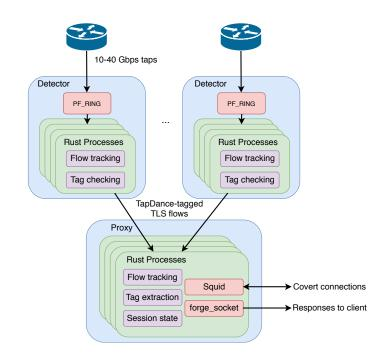
Figure 3.2: TapDance Station Architecture—Multiple detectors, central proxy
