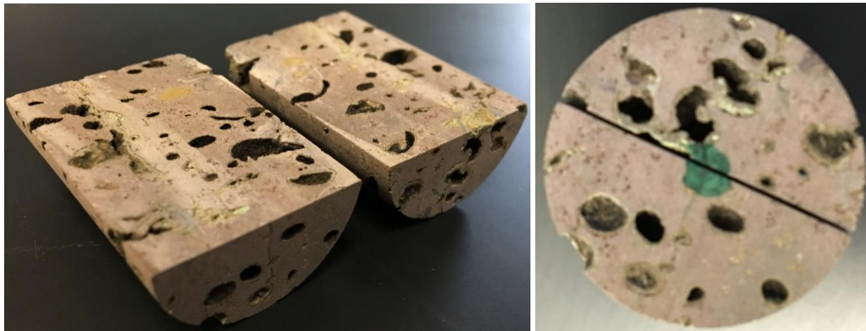
Figure F2. Grand Ronde core sample, illustrating the abundance of large vesicles.
