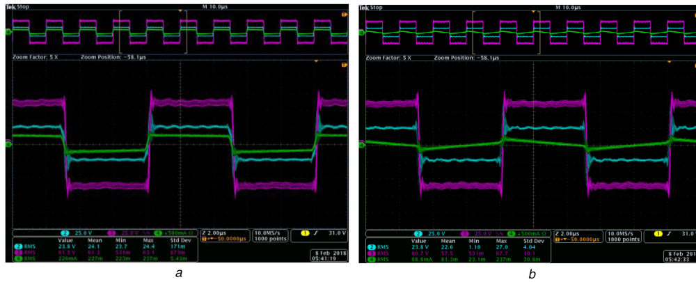
Fig. 15 Experimental voltage and current of the DAB transformer at different V_{in} and V_o (a) Phase-shift is zero, V_{in} \neq nV_o , (b) Phase-shift is zero, V_{in} = nV_o
