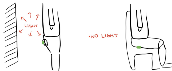
Figure 5.1 Mounting location of the photosensor on the participant
