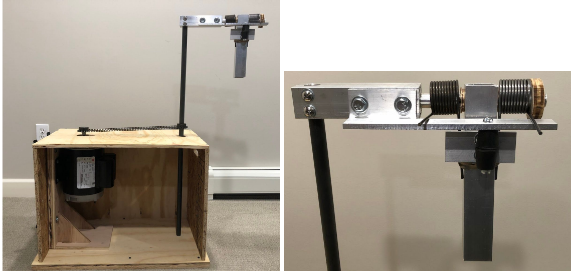
Figure 19: Our final assembled mechanism (left) and the detailed view of the upper arm and forearm linkage (right)
