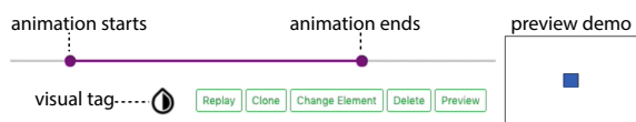
Figure 5.8: For each created animation, CoCapture provides information that prompts users about the actions they can take, including creating visual tags and replaying or previewing the animation. It also supports a set of operations to make the creation process easier and more accurate, including a range slider for time adjustment, as well as options for cloning, changing, or deleting an element.
