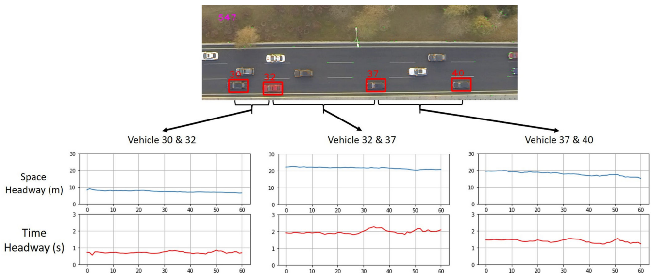
Fig. 9 Space headway and time headway extraction and car following behaviour analysis
