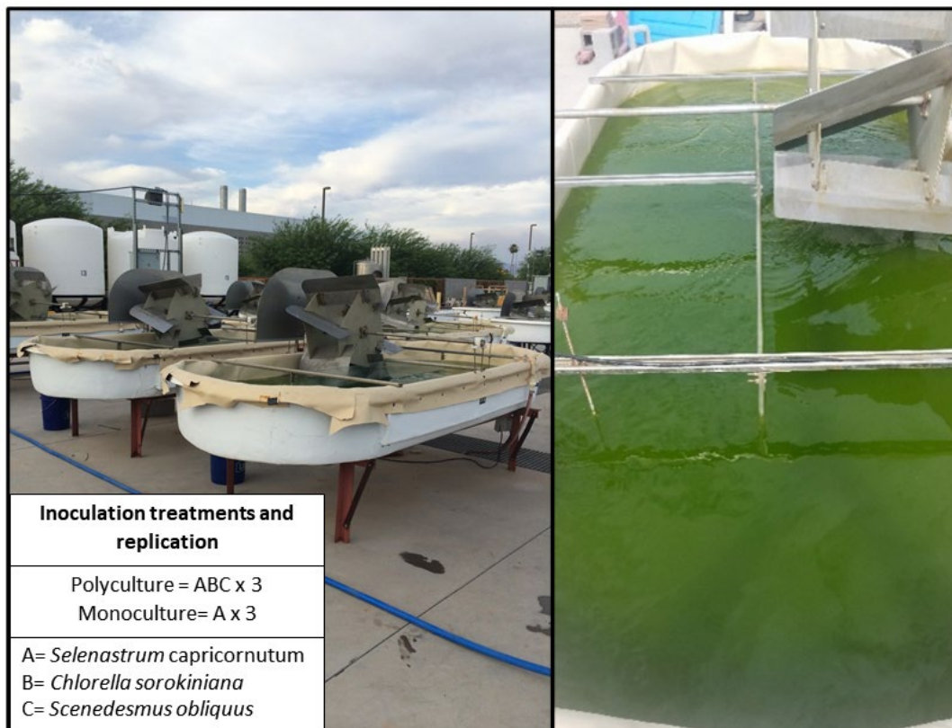
Figure 1. Photographs of 400 L experimental outdoor raceways located at Arizona Center for Algal Technology and Innovation (AzCATI) in Mesa, Arizona. Inset text summarizes experimental design.
