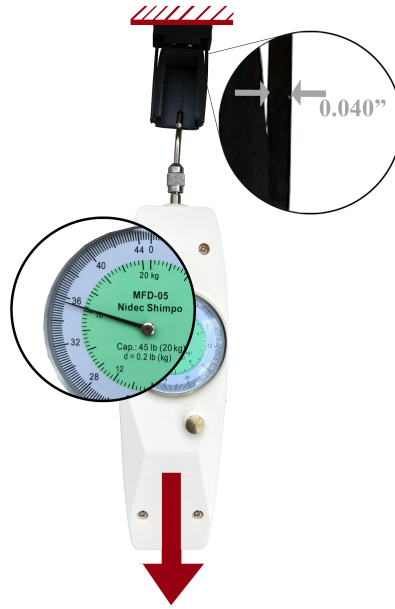
Figure 26. This figure shows a graphic representation of the tensile test conducted on the housing electrical interfacing components. The male buckle is mounted to the end of the tensile force gage connected to the female buckle grounded by a sufficient counter force. The close ups depict the max tension tested as well as a detail of the clasp arms of the buckle.
