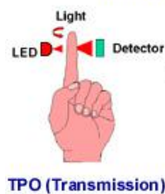
Figure 1. Transmissive Oximetry. A diagram of the mechanism for transmissive oximetry works on a finger. The LED passes light through the finger and the photodiode detects it on the other side [45].
