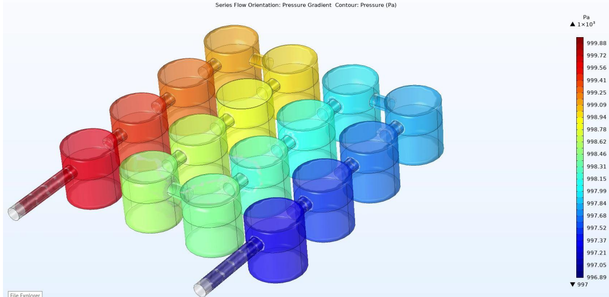
Figure 21: Media flow pressure gradient of the series media flow channel design. Inlet of the media flow is the left valve and outlet of the media flow is the right valve.
