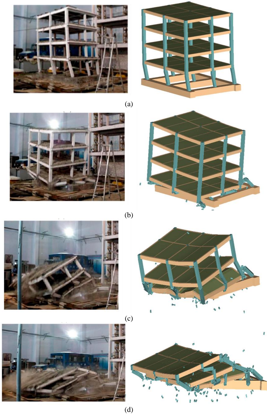
Figure 3-3 Comparison between experimental and numerical collapse progress at: (a) 0 s; (b) 0.858 s; (c) 1.155 s; and (d) 1.188 s (photos from Xu et al. 2017)
