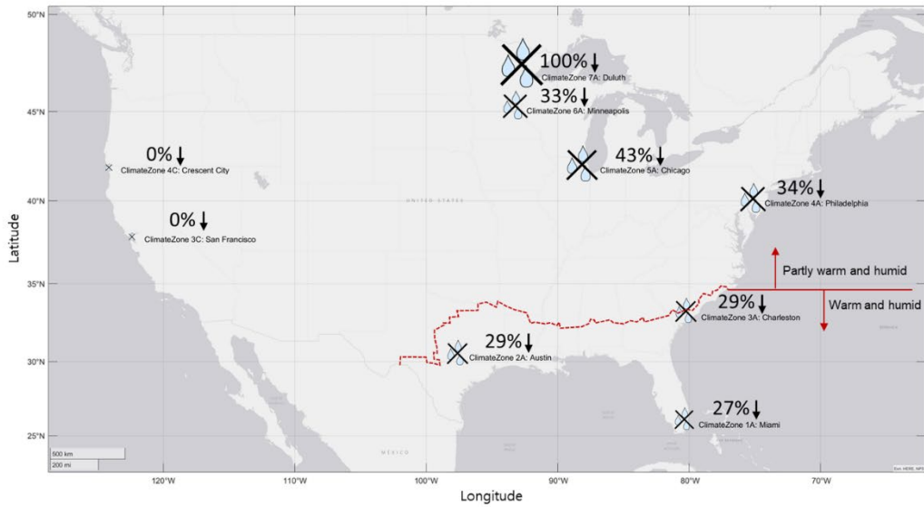
Figure 40. Site-specific surface condensation prevention performance (Geographic plot)
