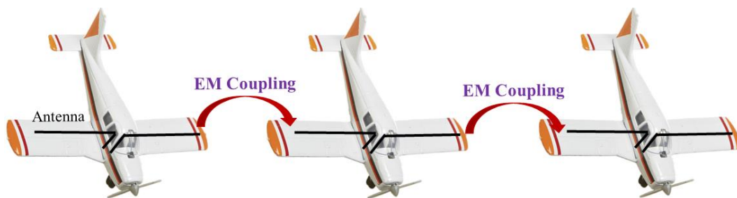
Figure 1.6. Concept of fragmented antenna formed by many electromagnetically-coupled small antennas on a cluster of UAVs.
