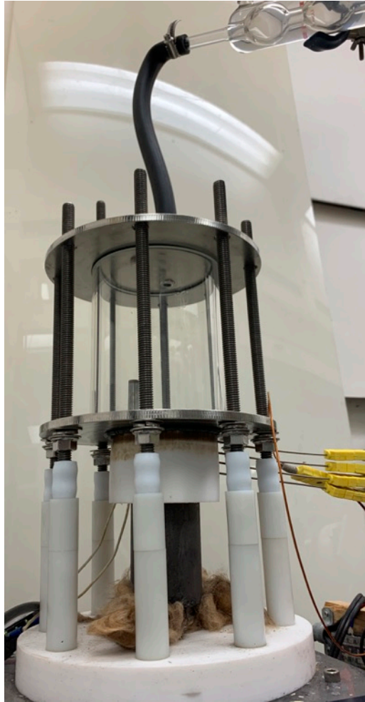
Figure 3.8: Image of the testing apparatus that was used for heat transfer measurements. The chamber containing the liquid is surrounded by a quartz cylinder between two stainless steel plates. The sample is inside this cylinder with the heat source embedded in copper and extending below the bottom plate. At the top is a tube leading to a condensation column that feeds the recondensed liquid back into the liquid chamber.
