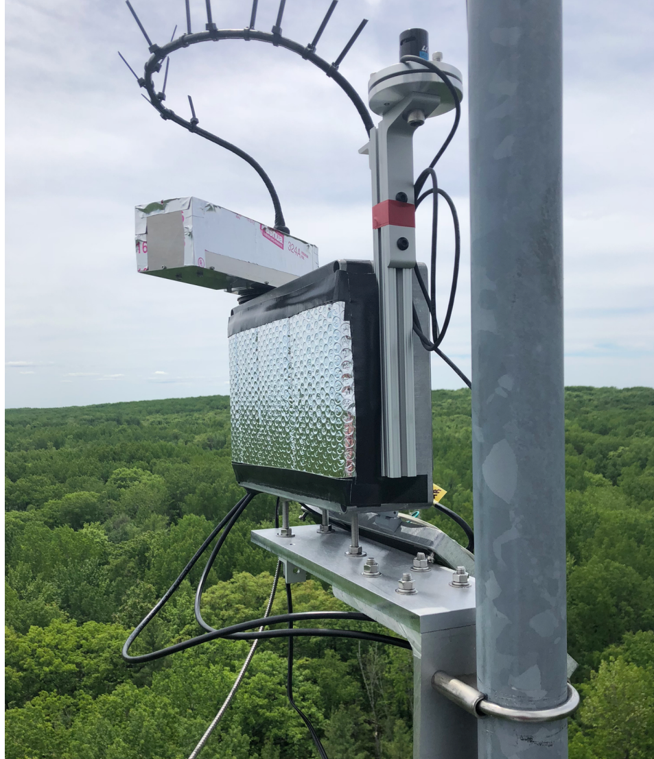
Figure A.4. PhotoSpec telescope unit attached to the US-UMB AmeriFlux tower.
