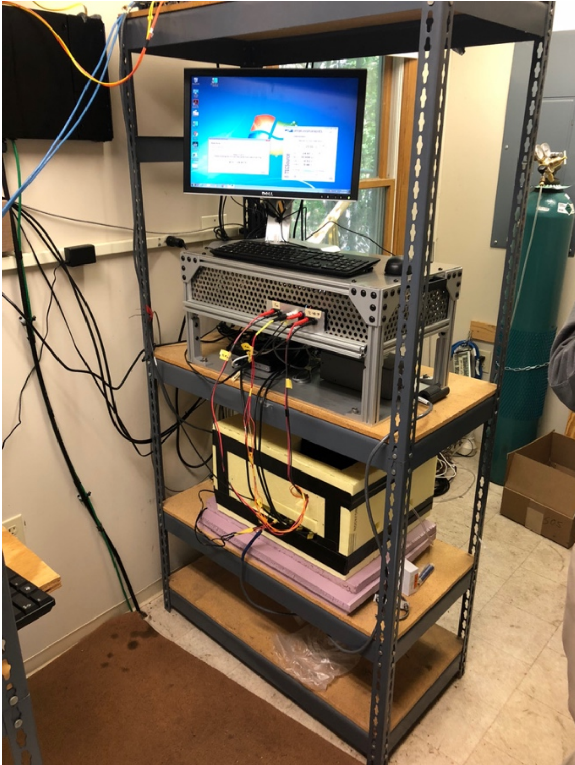
Figure A.2. Spectrometer housing and electronics at US-UMB. The computer, power supply, and temperature controllers are housed in the electronics box on the top shelf, while spectrometers are housed in the foam-encased enclosure on the lower shelf.
