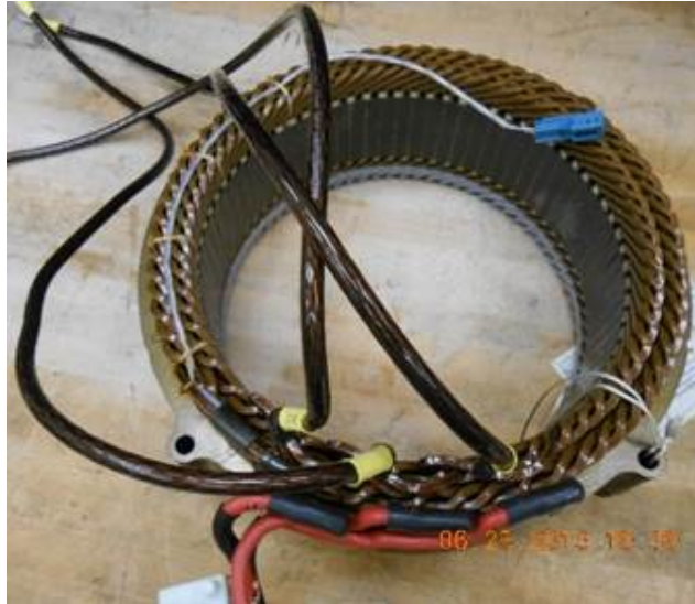
Figure 3.12: Stator with Rectangle Conductor Winding Provided by General Motors
