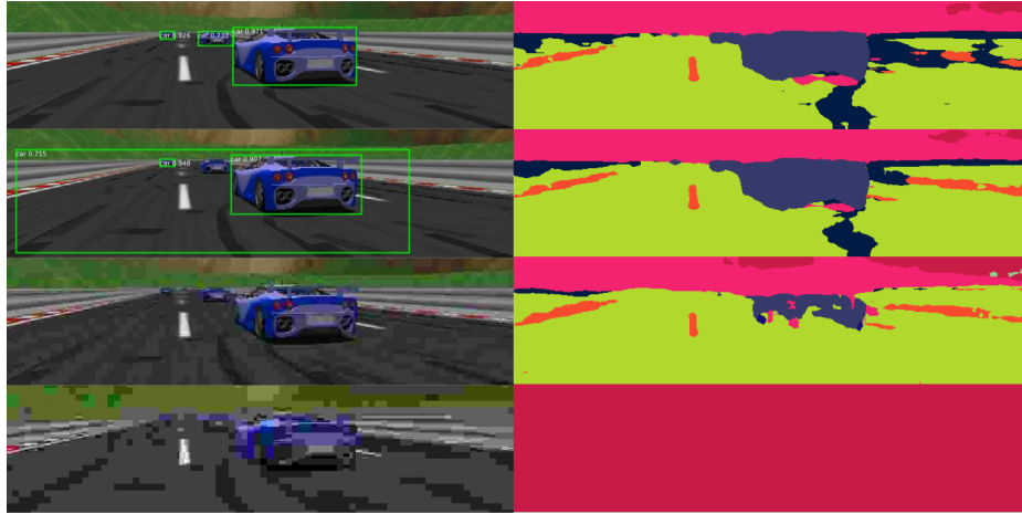
Figure 6.11: Object detection (left) and semantic segmentation (right) on a TORCS image compressed with 1, 0.5, 0.1 and 0.01 quality (from top to bottom).
