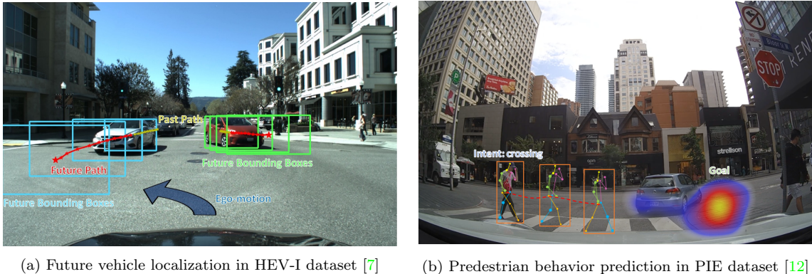
Figure 1.2: Understanding and predicting behavior of traffic participants is essential for autonomous driving systems. Typical tasks include but are not limited to (a) Vehicle trajectory prediction and (b) Pedestrian trajectory and intent prediction.
