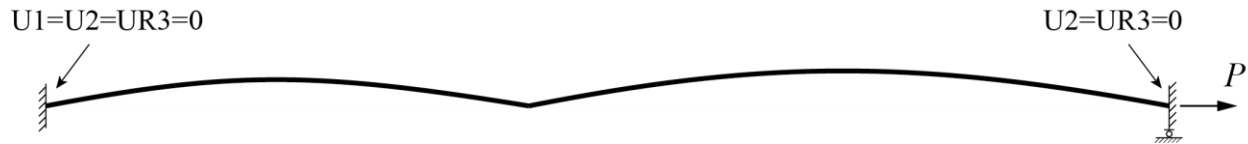
Fig. 4.5 Illustration of a representative FE beam model used for validation.
