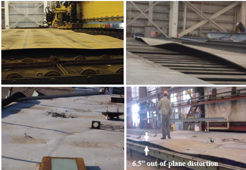
Fig. 1.5 Severe distortions associated with thin plates observed in shipyards [20].
