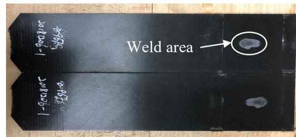
**Figure 2.7.** Illustration of weld area which is calculated by *ImageJ*
